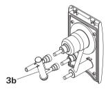
When the Ultraflow Filter Housing is to be used in conjunction with a Ultraflow Winter Kit (option – see page 5). Before connecting the blanked off end must be cut off.
