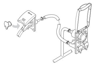
The blanking plug must be fitted to blank off the unused Compact or Filter system.
