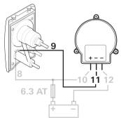
For the winter use, both housings must be connected directly to the Truma Smart Switch.
