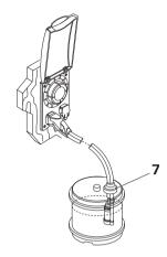
Place the pump into the water container, ensuring that it is fully submerged before operating the system. The dust cover (7) is to stop contaminates falling into the water container.
