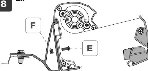
**EN** Before tightening the screws, make sure that the awning position doesn't prevent the opening of the rear door.
