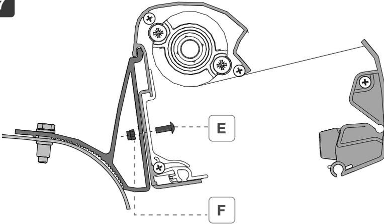
**EN** Before tightening the screws, make sure that the awning position doesn't prevent the opening of the rear door.
