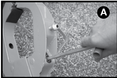
A. Using the hex tool, unscrew the hex bolt anti-clockwise to open the 'jaws'.
