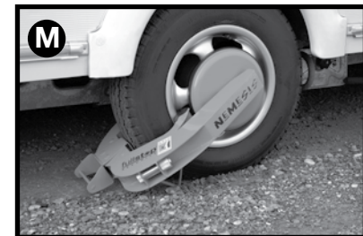
M. Remove the key and your wheel clamp is now fitted. Two keys are provided. Please keep the keys in a safe, secure place.
