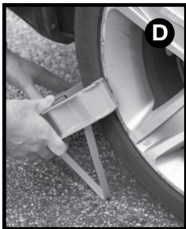
D. The tips of the 'jaws' should be fitted into the wheel as far as possible. A little experimentation will be required to ensure a secure fit for your application.
