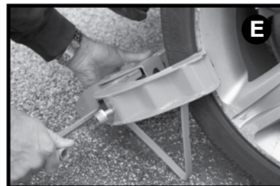
C. Fit the 'jaw' section around the wheel.
