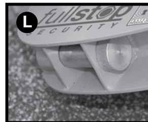
L. Insert the female lock portion into the apertures of the lock cradle on the wheel cover arm. Insert the male lock portion into the female lock portion and secure with the key.
