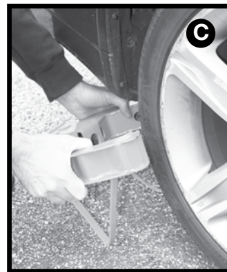
C. Fit the 'jaw' section around the wheel.
