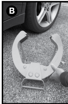
B. Check that the 'jaws' open enough to fit around the tyre.
