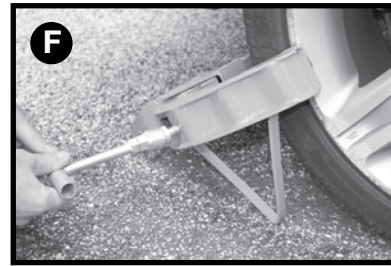
F. If necessary, unscrew (by turning anti-clockwise) the securing hex bolt for the wheel cover arm. Do not fully remove.
