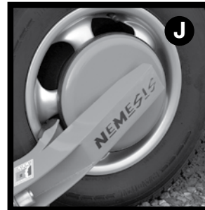
J. Hold the arm in position. The round wheel cover has a slide and tilt mechanism and should be adjusted to be central to the face of the wheel as much as possible. On larger wheels where central location is not possible, it must be ensured that at least one of the wheel nuts is covered.
