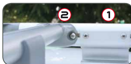
(1) Roof Rail supporting brackets (2) Fixing-Bar Rail terminal.
