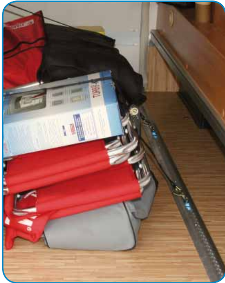
Model 60 is standard delivered with 2 click strips for the fixing of the scooters.
