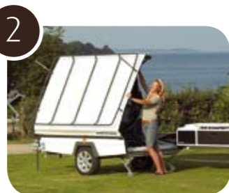
2 The gas assisted opening helps you open the lid.
