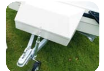
Gas and water box.
