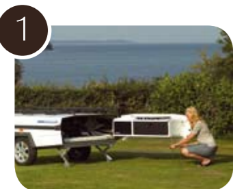
1 Wind down the support legs and swing out the kitchen.
