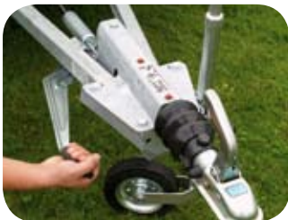
Road and hand brake for additional security. Jockey wheel for easier transportation.
