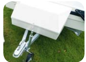
Gas and water box.
