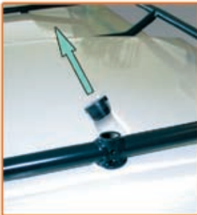
Remove the plastic stoppers from the luggage rack (keep the stoppers in a safe place).
