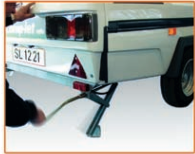
The rear supporting legs has to be screwed down and adjusted, so that the trailer stands horizontal in both directions. The supporting legs must be screwed down so the wheels nearly lets go of the ground. Unlock the Camp-let.
