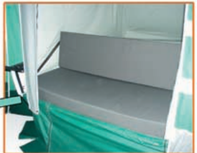
The back rest strap goes through the inner tent then hooks onto the ring. Replace the mattresses.
