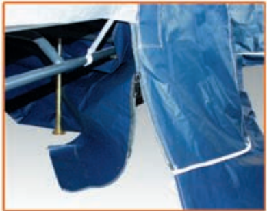
Apollo/Lux: Fitting the bottom skirt. Savanne/Concorde: Fitting the bottom skirt with under bed storage. Zip the skirt to the canvas on both sides before you do the press-studs.
