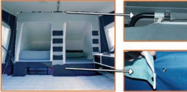
Mounting the pelmet with pockets. (Standard in Savanne/Concorde).
