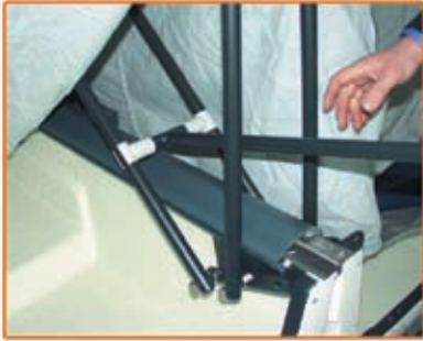
Savanne/Concorde: Before mounting the wardrobe bar, check the awning canvas is sitting correctly on the 4 corners of the roof.
