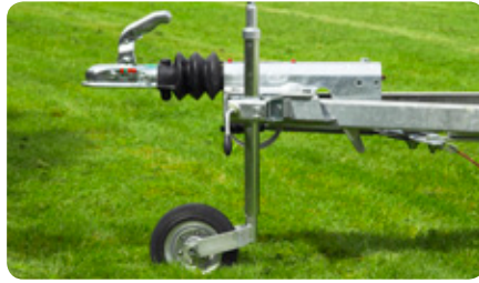
Jockey wheel | For easy handling, and to enable easy manoeuvring of the Camp-let into tight spaces.
