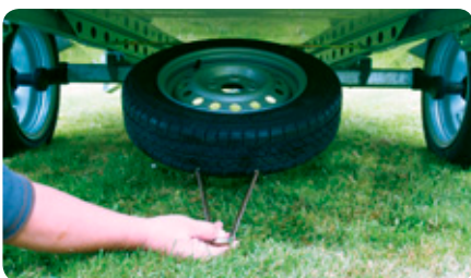
Spare wheel and carrier | Practical under-trailer mounting.
