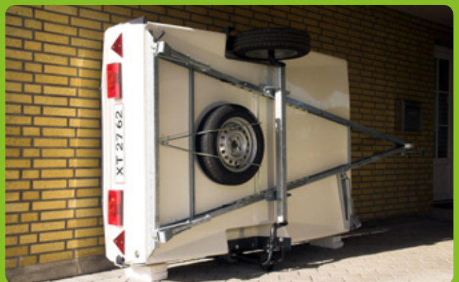
Storage after your holiday | Using a storage bracket, the trailer is put upright and can be pushed into the garage. For details of the storage bracket, see optional extras.
