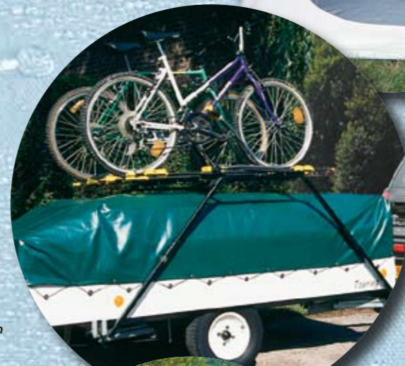
Carry rack - max. Carrying capacity 45kg. Cycle brackets etc not included.
