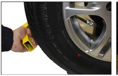
**4.** Pass the rear arm around the rear of the wheel and position the locking bar through the aperture of the wheel.
