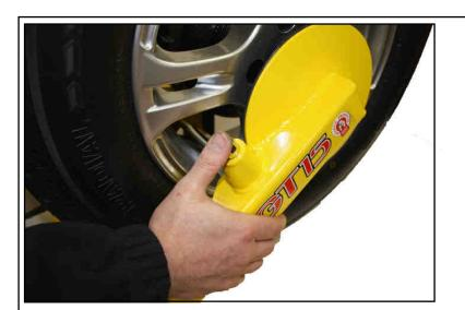
**6.** Push the lock down to lock the clamp in place.
