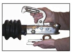
1. Insert dummy ring plate. If hitch handle is in raised position the plate can be used to release handle.
