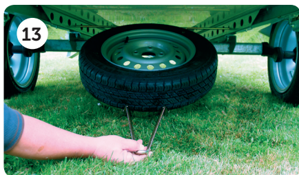
13 Spare wheel and carrier | Practical under-trailer mounting.
