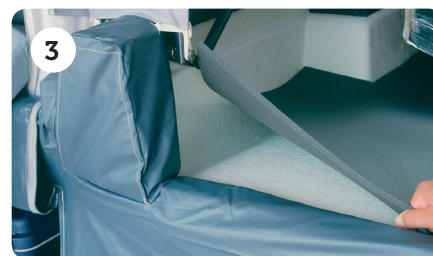
3 Insulation mats | Extend the season with extra insulation beneath the mattresses.
