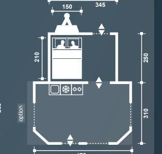
**EN** Total laden weight : 650 kg ■ Unladen weight : 400 kg, 460 kg with kitchen unit ■ Mechanical brakes : standard ■ Size of wheels : 165/70 R13 ■ Size of the body (LxHxW) : 435 x 171 x 105 ■ Total area : 8,6 m<sup>2</sup> ■ Suspension : rubber with independant wheels with shock absorbers
