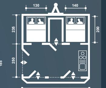
**EN** Total laden weight : 650 kg ■ Unladen weight : 465 kg with kitchen unit ■ Mechanical brakes : Standard ■ Size of wheels : 135 R 13 ■ Size of the body (LxHxW) : 383 x 162 x 120 ■ Total area : 25,7 m<sup>2</sup> ■ Suspension : Rubber with independant wheels
