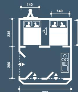
**EN** Total laden weight : 650 kg ■ Unladen weight : 365 kg with kitchen unit ■ Mechanical brakes : Standard ■ Size of wheels : 135 R 13 ■ Size of the body (LxHxW) : 383 x 162 x 105 ■ Total area : 18,9 m<sup>2</sup> ■ Suspension : Rubber with independant wheels
